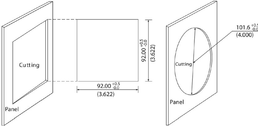
2. Remove the clips from the meter and insert the meter into the square hole from the front side. Please note: optional rubber gasket must be installed on the meter before inserting the meter into the cut out.
