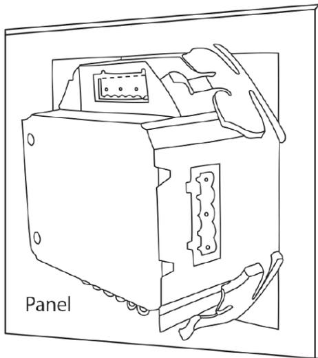
**NOTE** The display meter and the remote display unit have the same installation method. The DIN rail meter is simply installed on a 35mm DIN rail.
