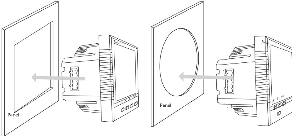
3. Install clips on the back side of the meter and secure tightly to ensure the meter is affixed to the panel.
