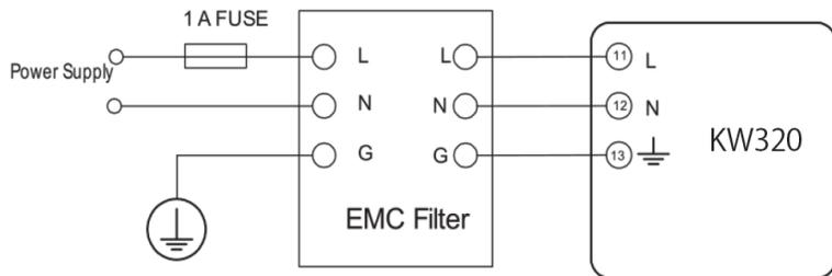
Choice of wire of power supply is AWG 22-16 or 0.6-1.5 mm<sup>2</sup>.
