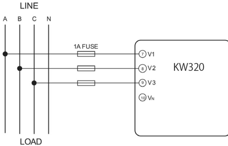
Figure 3: 3LL 3-Phase 3-Line Direct Connection
