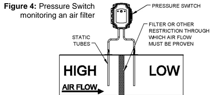
To set the pressure trip point, remove the tubing from the Pressure Switch. Connect a manometer and a pressure source to the high pressure port on the Pressure Switch. Use the manometer to measure the pressure. Set the pressure as described in the *Proper Adjustment Procedures* section above. Reconnect tubing when finished.
