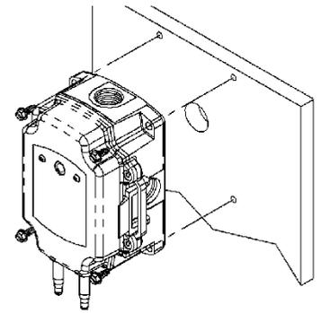
**Figure 2:** Differential Pressure Switch Mounting
