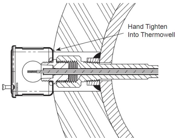
Typical Sensor Inserted
