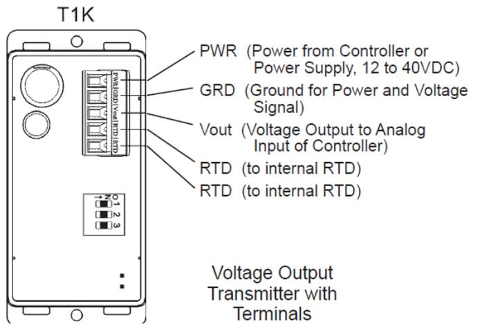
DIP Switch Settings for Field-Selectable Output
