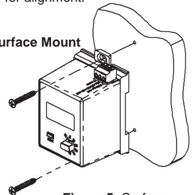
Figure 5: Surface mounting with the tabs out.
