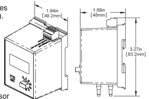
Figure 1: Low Pressure Sensor
