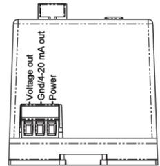
Figure 7: Wiring terminations
