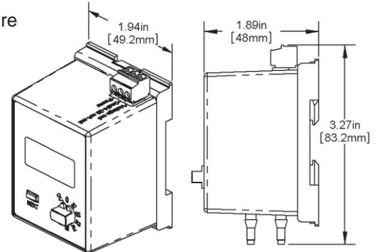
Figure 1: Pressure Sensor
