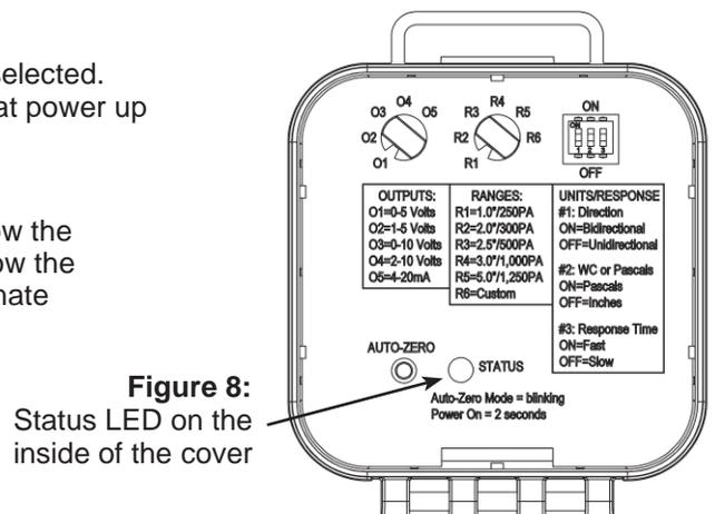
Figure 8: Status LED on the inside of the cover
