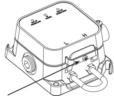
A locking screw can be inserted into the hole in the cover latch to prevent unintentional cover openings.
