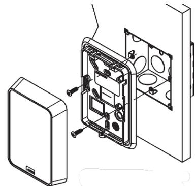
Figure 2: European wall box mounting with 60mm base
