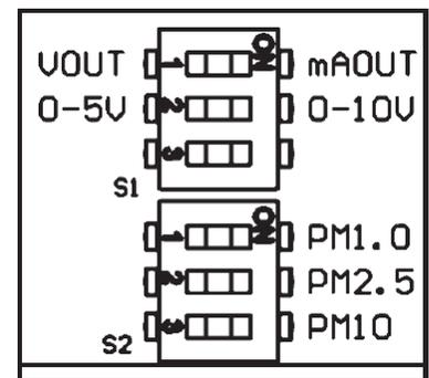
Figure 5: DIP Switches S1 and S2
