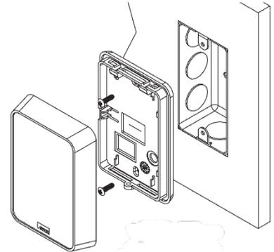
Figure 1: Jbox Mounting with Standard Base
