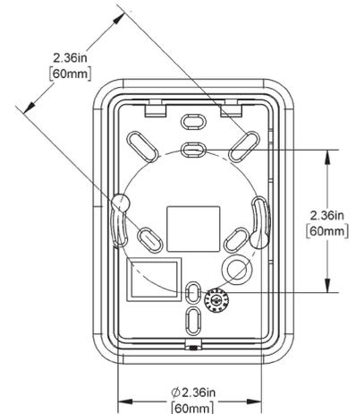
Figure 3: 60mm mounting base dimensions
