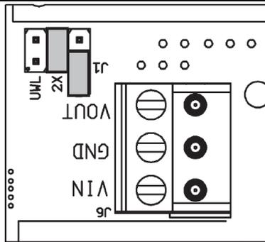
Figure 5: J1 set for 0 to 10 VDC output
