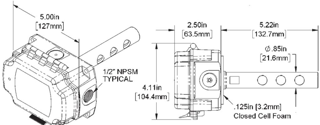
Figure 1: Duct VOC Sensor
