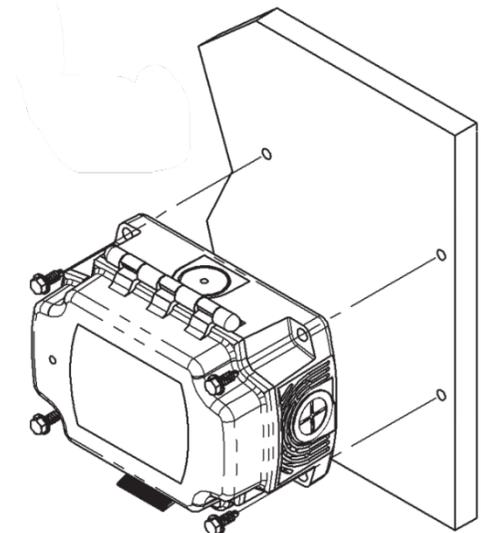
Figure 3: Rough Service Unit Mounting
