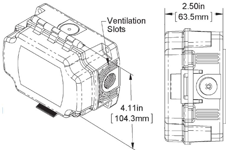
Figure 2: Rough Service VOC Sensor
