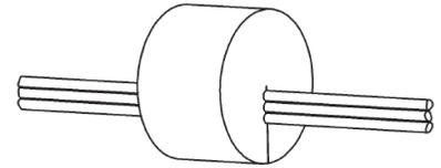
Figure 7: Wires Through Foam Plug
