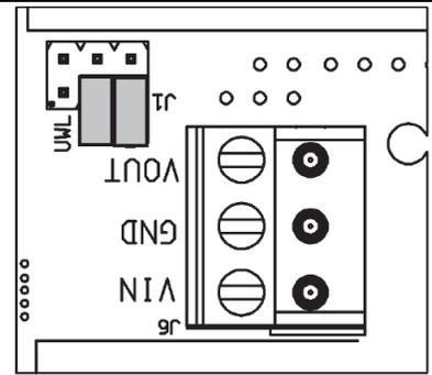
Figure 6: J1 set for 0 to 5 VDC output
