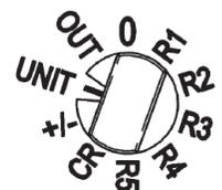
Figure 7: Rotary Switch Position for Unit Mode Selection
