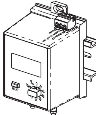
Figure 1: DIN Rail Mounting with Tab Out
