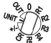
Figure 7: Rotary Switch Position for Unit Mode Selection
