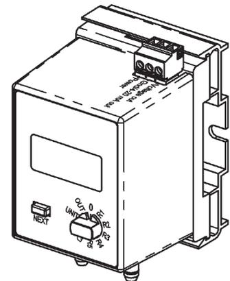
Figure 4: Snaptrack Mounting with Tabs In
