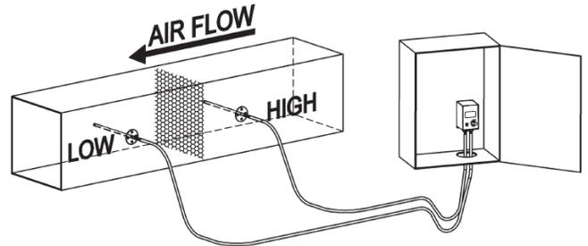
Figure 8: Air filter pressure drop monitoring with the EZ Low Pressure Sensor mounted in a panel with two static pressure probes
