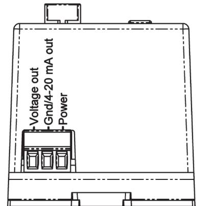
Figure 6: Wiring Terminations
