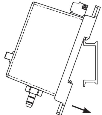
Figure 2: Catch the EZ mount hook on the edge of the DIN Rail, then rotate into place
