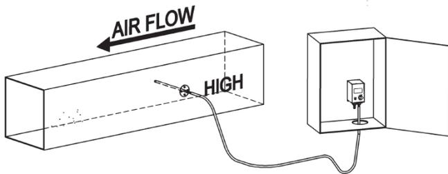
Figure 9: Duct static pressure monitoring with the EZ Low Pressure Sensor mounted in a panel with a static probe in the duct
