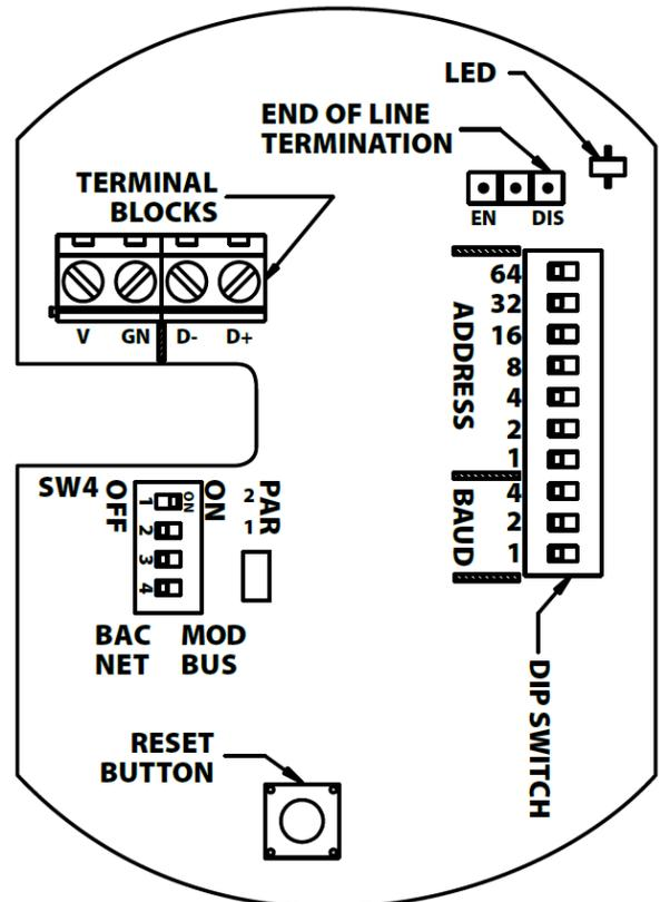
Figure 3: Wiring Diagram
