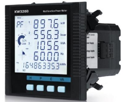
Active Power, Reactive Power and Apparent Power – see table 1 for all parameters monitored and metered. Current input are compatible with a 333mV and Flexible Rogowski Coil CT. Meters come standard with a three channel CT input to accurately measure neutral current. CTs are sold separately as shown on the Split-Core, Solid-Core and Rogowski Current Transformer product data sheets.
